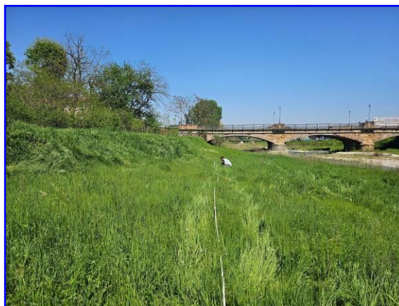
Microsismic e stendimento MASW
