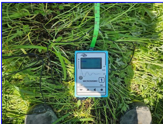
Microsismic e stendimento MASW
